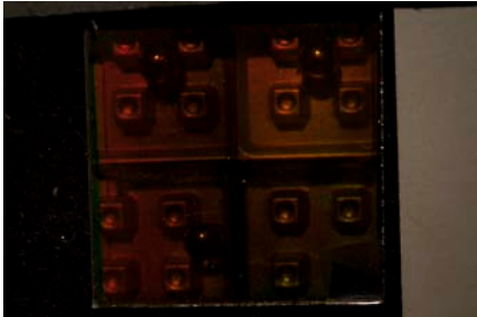
#139: Harman Red, 800, 1600, 3200, 6400 \mu\text{J}/\text{cm}^2 at 633 nm, 2' Pyrochrome Developer and Bleach. Cut from a 30 by 40 cm.
