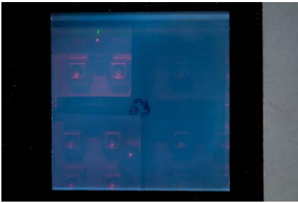
#53: Agfa 8E75HD, erased, 50, 100, 200, 400 \mu\text{J}/\text{cm}^2 , 30" BBAA, some dim noisy images, but maybe it seems that this is not a good developer for this material.
