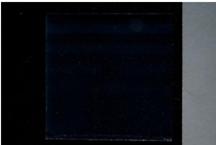
#47: PFG-03M, 200, 400, 800, 1600 \mu\text{J}/\text{cm}^2 , 1' BBAA, totally blank. Must really need the low alkalinity of the GP-2.
