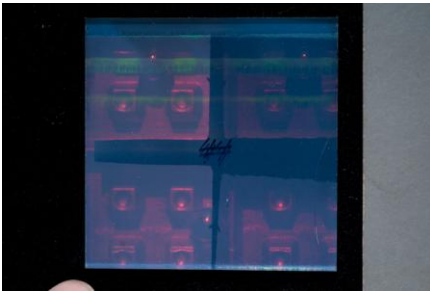
#44: Slavich PFG-01, 50, 100, 200, 400 \mu\text{J}/\text{cm}^2 , 1' BBAA, looks fogged but an image is still there.
