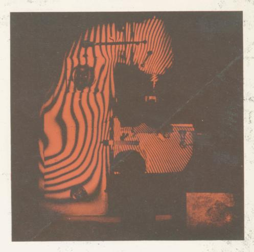
A milling-machine has been loaded. Each interference fringe corresponds to a movement of 0.3 µm. Dense fringes signify a big movement. Straight
