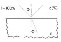
$$R = \frac{1}{2} \left[ \frac{\sin^2(\Phi - \Phi')}{\sin^2(\Phi + \Phi')} + \frac{\tan^2(\Phi - \Phi')}{\tan^2(\Phi + \Phi')} \right]$$
