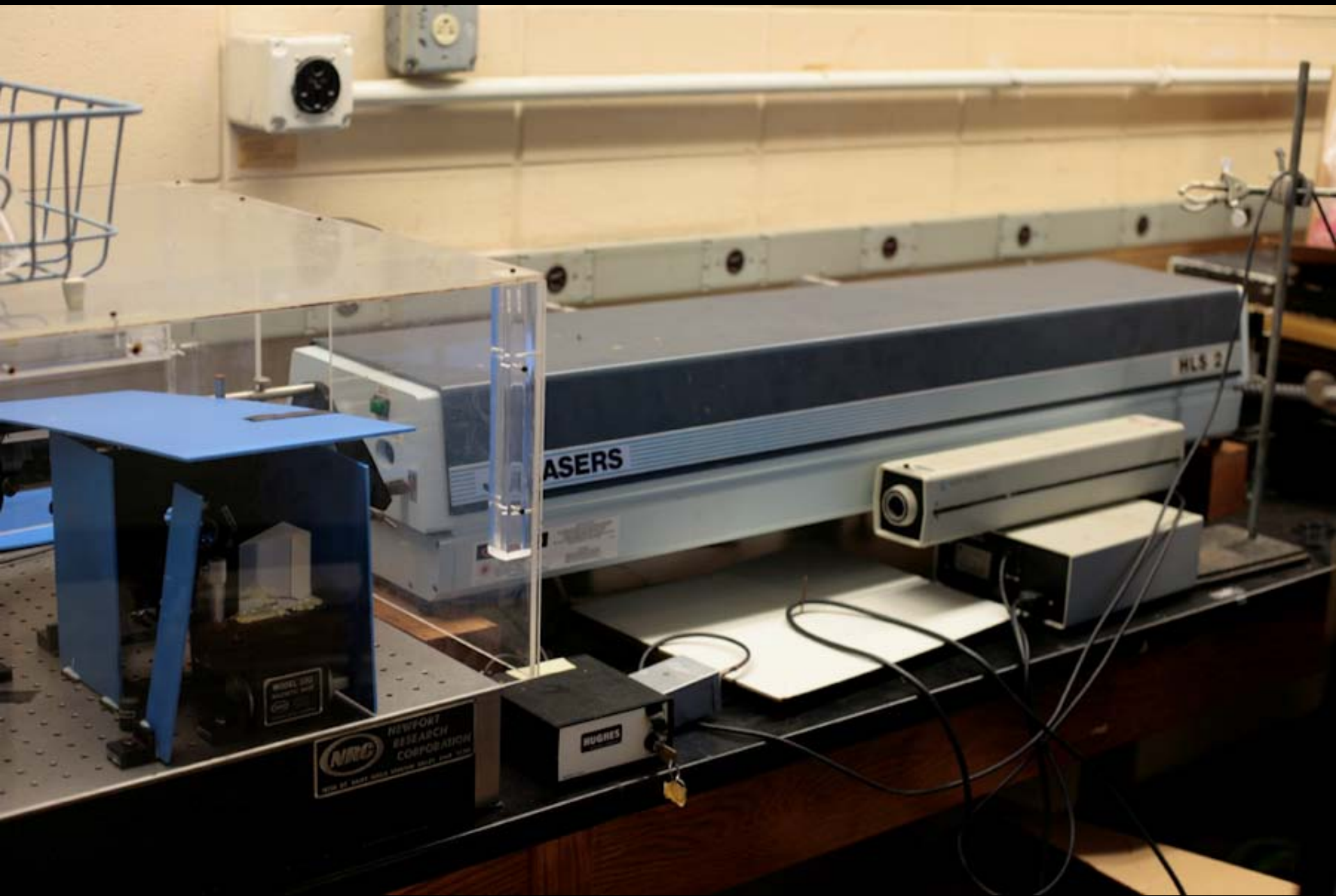
HLS-2 feeds into optics on Newport mini table
