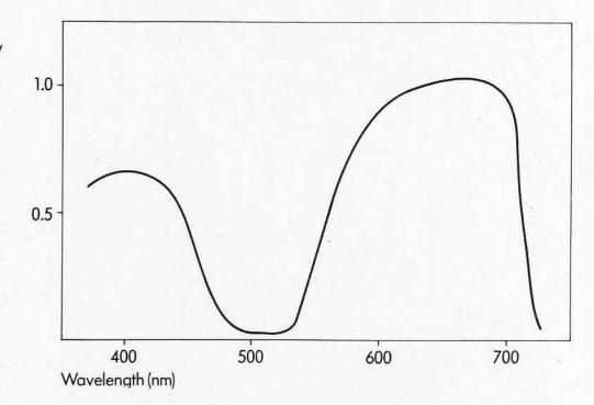
The above curve shows the relative spectral sensitivity of SP673 holographic film to white light flash exposure  $(10^{-4}\text{s})$ . This curve shows that SP673 holographic film has high sensitivity at 633nm, 647nm and 694nm as well as in the blue region of the spectrum.
